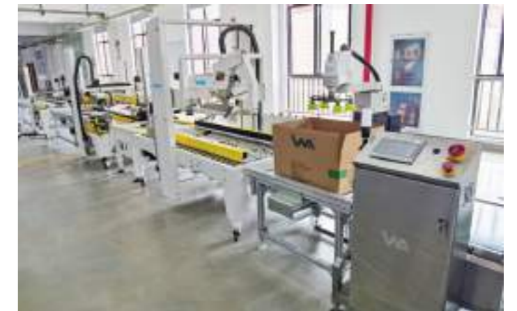
自动称重、封箱、捆扎 Automated weighing, sealing, and strapping
