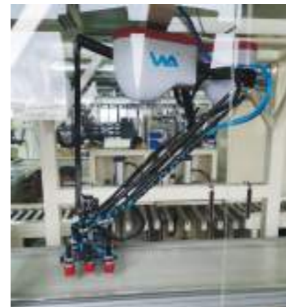
并联机器人分拣入箱 Parallel robot sorting and packing
