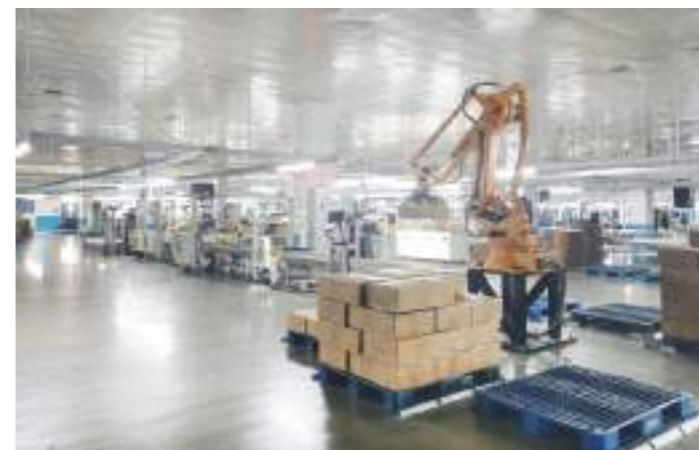
机械手臂自动码垛 Mechanical arm automatic stacking
